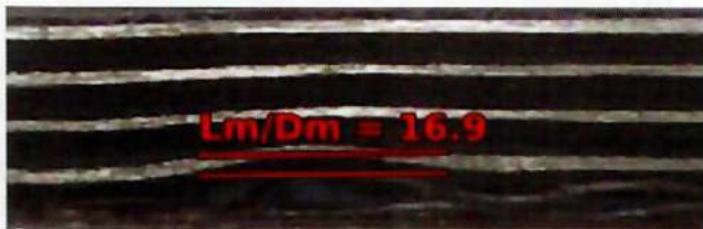
Figure 3 – Example of wrinkle severity annotation
