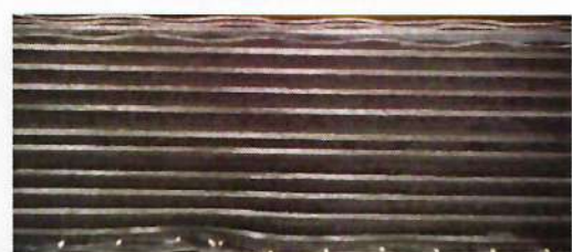
Figure 9 – Incorrect detection of last ply. Wrinkle severity Figure is not performed in this case
