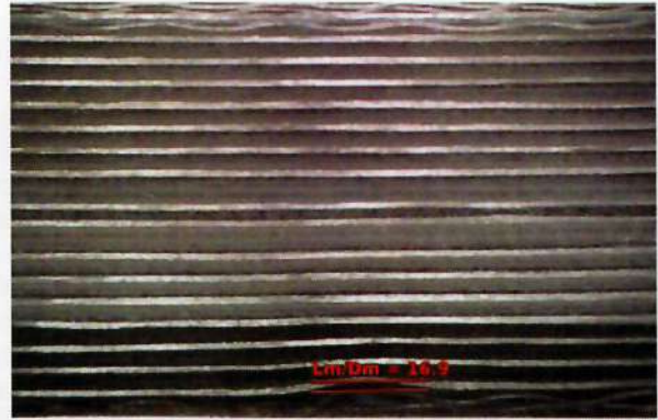
Figure 6 – Correct measurement of the wrinkle severity figure
